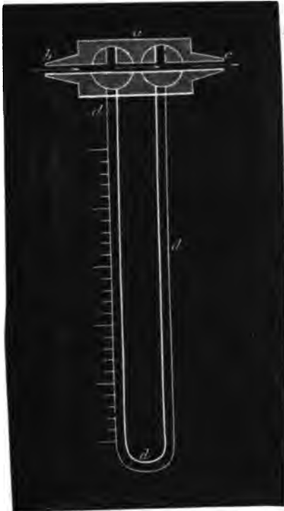
VOLKMANN'S APPARATUS for measuring the rapidity of the arterial circulation.
